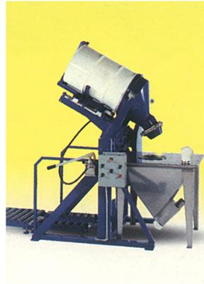
Lift, seal, and unload drums dust-free
